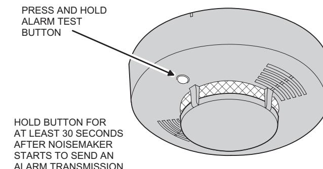
**STEP 9 Complete receiver programming.** Refer to the instructions supplied with the supervised receiver to program the TSD-90A as a 24-hour fire alarm. Repeat the previous step to verify that the TSD-90A triggers the correct zone on the receiver and that the correct report is sent to the central station (if the system is monitored).
